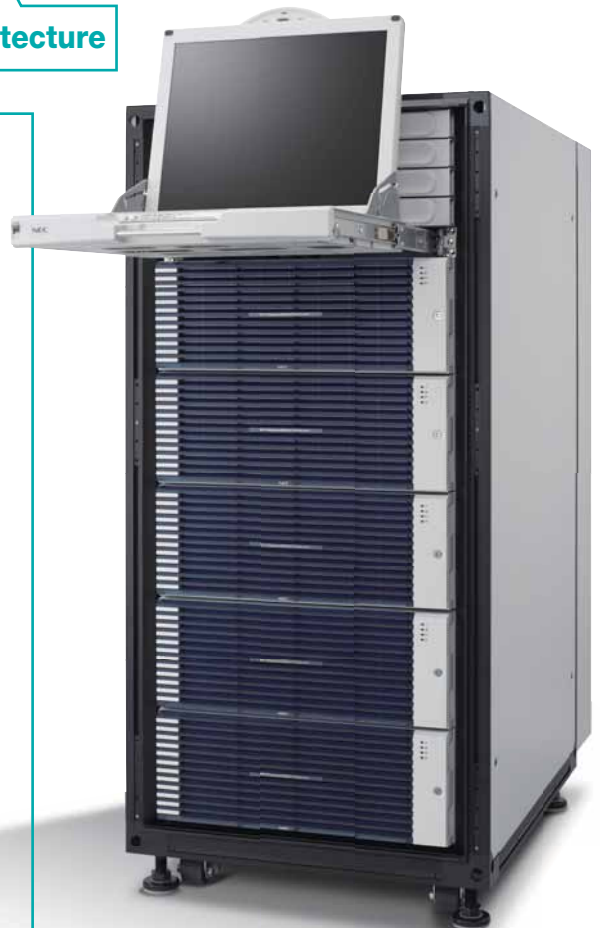
Disk drives are built into each module. Rapid Disk Resync (RDR) ensures disk redundancy.
