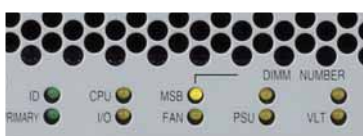
EXPRESSSCOPE LED indicators allow users to visually identify failed components
